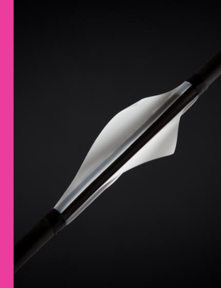
The "Shark" Vane profile have the free tip to wrap around themselves during the first phases of flight and, following the heeling of the arrow, they open giving a greater deporting surface useful to give a more rapid stabilization of the shaft. When the arrow takes its correct direction of flight, the Shark vane tend to close on themselves in order to offer a smaller surface and, therefore, less friction to the advantage of the speed of the arrow.
